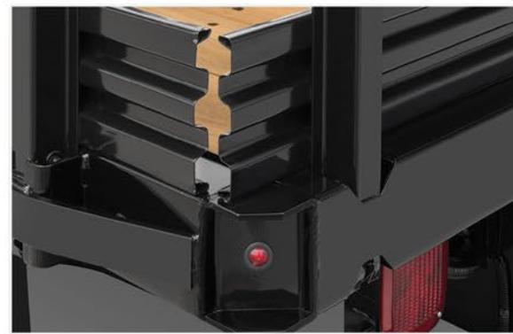
Heavy-duty Apitong wood flooring comes standard on all ProStake bodies, and offers natural shock absorption, weather and insect resistance.
