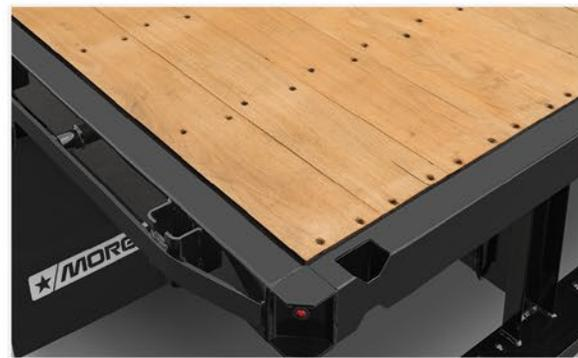
A standard, heavy-duty rub-rail helps to protect the flatbed frame and side rail pockets from minor impacts.
