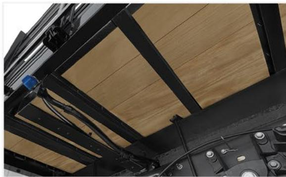
The use of bulkhead gussets helps to reinforce strength for enhanced durability, and transfer stress for greater longevity.
