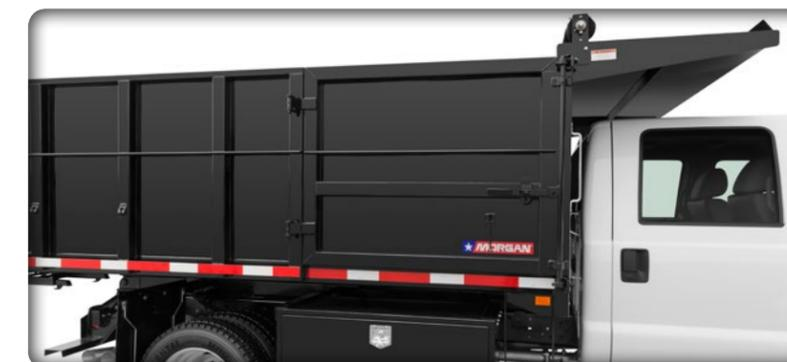
Side Door at curbside foremost location to swing towards rear with cam action lock hardware and door hold backs.
